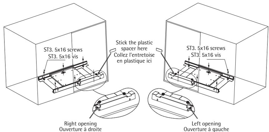
**Step 3: Connect the frame and bottom base with hexagon screws.**
