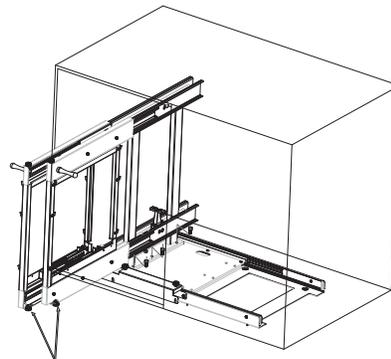
NOTE: Left opening, the right wheel is installed into the oval hole, the left wheel is installed into the round hole.
