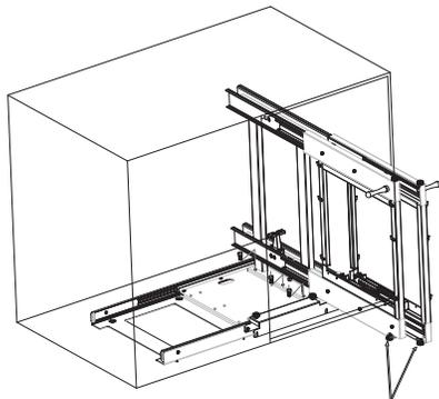
NOTE: Right opening, the right wheel is installed into the round hole, the left wheel is installed into the oval hole.
